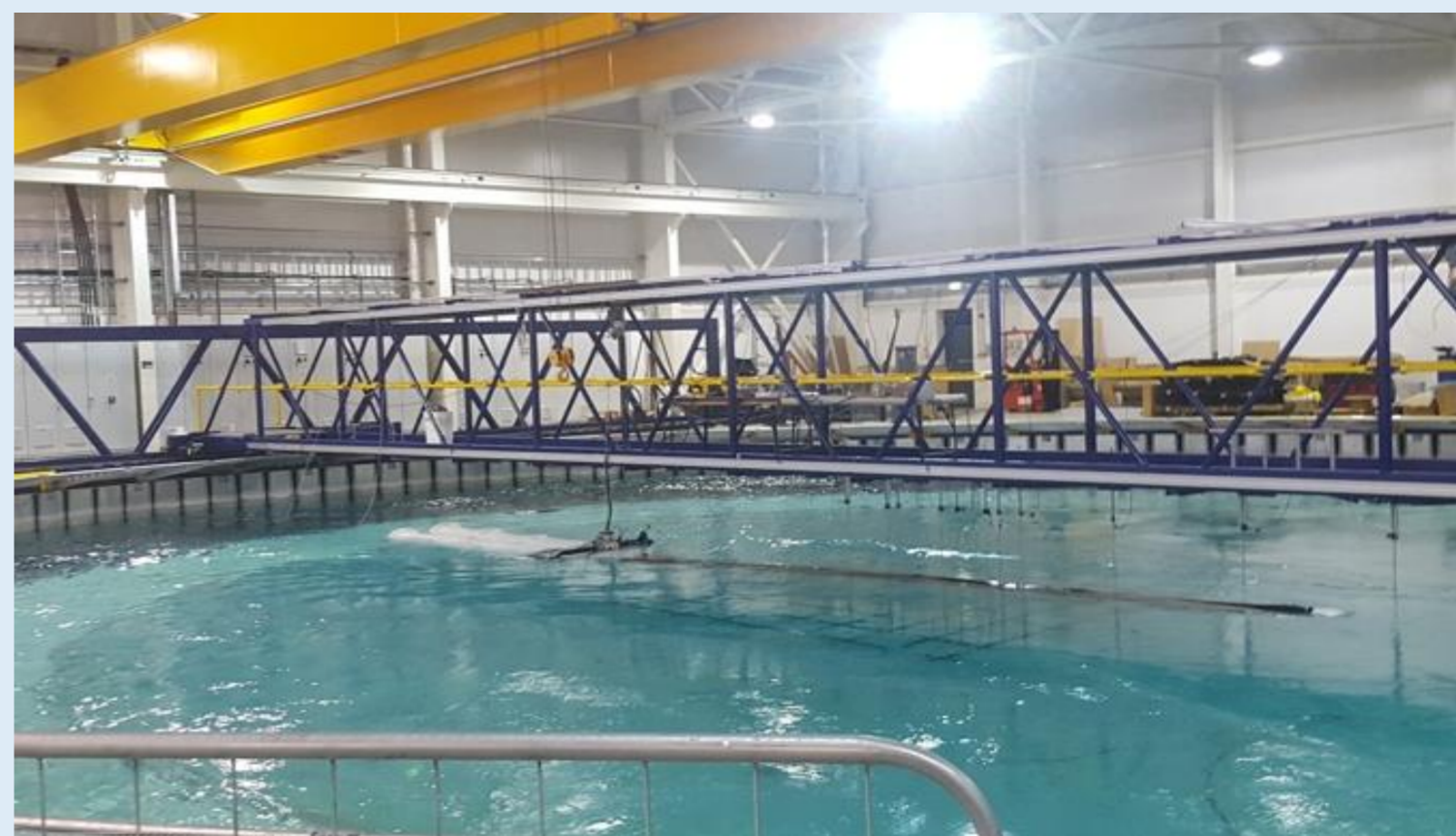
Anaconda Mk1 under test at Flowave TT
