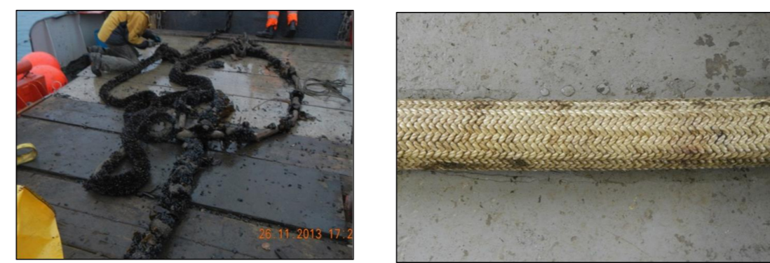
Figures 4 & 5: Marine growth on Tether P1-8. Before (L) and after (R) cleaning
