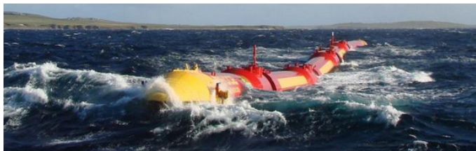
One of the two Pelamis P2 machines currently based in Orkney
