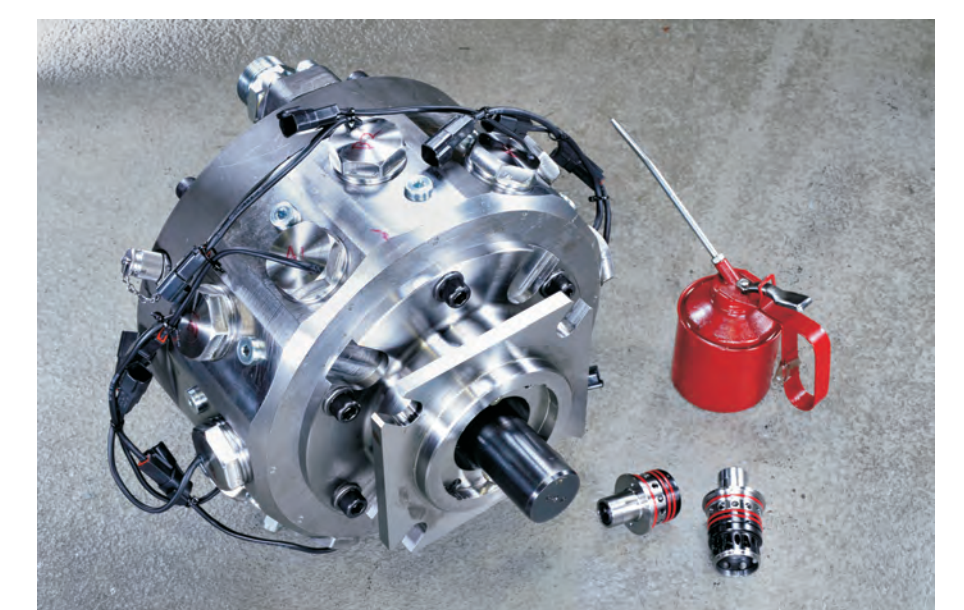
Left: Block diagram illustrating the Quantor PTO concept. Right: Artemis 'M96' Digital Displacement pump-motor DDPM specially developed during the project.
