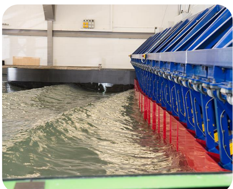
Figure 2. Generating off-angle waves in Portaferry wave tank
