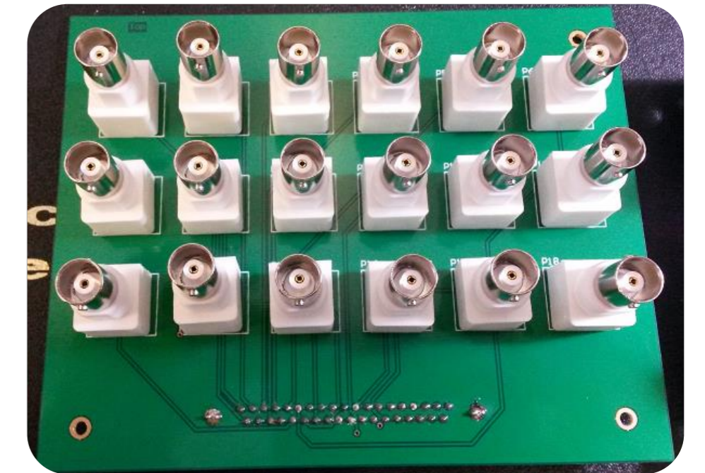
Figure 5. Data acquisition system developed for Portaferry wave tank
