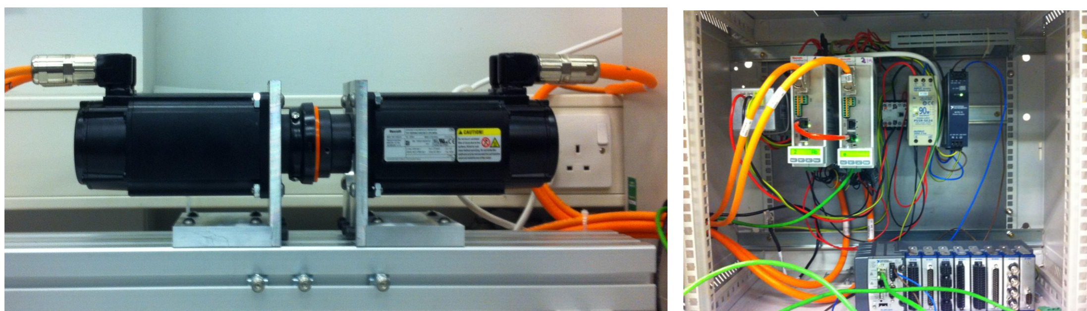
Figure 3: Instrumented Drive Train Test Rig.
