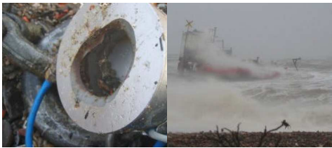
Fig. 1: Stranded Wavedragon due to broken force transducer [2, p. 17]
