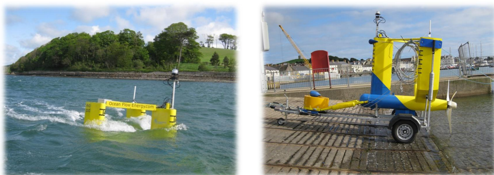
Figure 1 – Evopod tidal energy device
