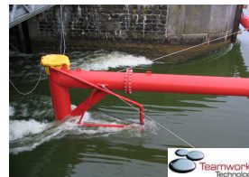
Fig. 2 Artificial drag element in channel - free surface. Fig. 3. Sample velocity reduction along channel in wake of tidal energy device. After Bryden et al. (2006) 2 .
